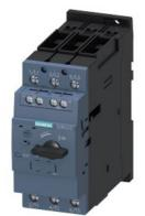
Circuit breaker size S2 for motor protection class 20 A-release 12...17 A N-release 260 A screw terminal Standard switching capacity with transverse auxiliary switch 1 NO+1 NC  $\,$
