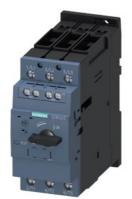
Circuit breaker size S2 for motor protection, CLASS 10 A-release 28...36 A N-release 520 A screw terminal Standard switching capacity with transverse auxiliary switches 1 NO+1 NC
