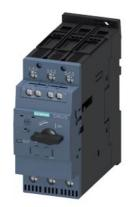
Circuit breaker size S2 for motor protection, CLASS 10 A-release 54...65 A N-release 845 A screw terminal Standard switching capacity with transverse auxiliary switches 1 NO+1 NC
