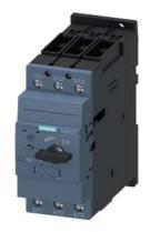
Circuit breaker size S2 for motor protection, CLASS 10 A-release 22...32 A N-release 416 A screw terminal Standard switching capacity
