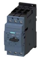
Circuit breaker size S2 for motor protection, Class 20 A-release 18...25 A N-release 325 A Screw terminal Standard switching capacity
