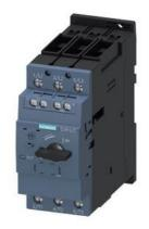
Special type Circuit breaker size S2 for motor protection, Class 10 A-release 14...20 A Short-circuit release 260 A Screw terminal Standard switching capacity with transverse auxiliary switches 1 NO+1 NC Ambient temperature -50 °C 250 switching cycles
