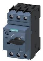
Special type Circuit breaker size S0 for motor protection, CLASS 10 A-release 34...40 A N-release 480 A screw terminal Standard switching capacity Ambient temperature -50  $^\circ$ C 500 switching cycles
