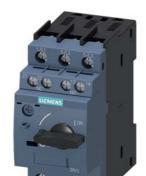
Special type Circuit breaker size S0 for motor protection, CLASS 10 A-release 27...32 A N-release 400 A screw terminal Standard switching capacity with transverse auxiliary switches 1 NO+1 NC Ambient temperature -50 °C 500 switching cycles
