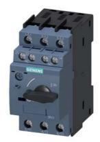
Circuit breaker size S0 for motor protection, CLASS 10 A-release 10...16 A N-release 208 A screw terminal Standard switching capacity with transverse auxiliary switches 1 NO+1 NC
