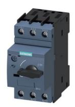
Circuit breaker size S0 for motor protection, CLASS 10 A-release 10...16 A N-release 208 A screw terminal Standard switching capacity Multi-unit packaging Pack = 12 units
