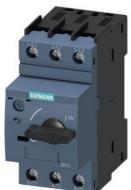
Circuit breaker size S0 for system protection without phase failure protection Arelease 10...16 A N-release 208 A screw terminal Standard switching capacity
