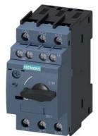
Circuit breaker size S0 for motor protection, CLASS 10 A-release 7...10 A N release 130 A screw terminal Standard switching capacity with transverse auxiliary switches 1 NO+1 NC  $\,$
