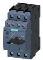
Circuit breaker size S0 for motor protection, CLASS 10 A-release 3.5...5 A N release 65 A screw terminal Standard switching capacity with transverse auxiliary switches 1 NO+1 NC  $\,$
