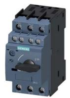
Circuit breaker size S0 for motor protection, CLASS 10 A-release 2.8...4 A N release 52 A screw terminal Standard switching capacity with transverse auxiliary switches 1 NO+1 NC  $\,$
