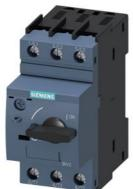
Circuit breaker size S0 for motor protection, Class 10 A-release 0.11...0.16 A Short-circuit release 2.1 A Screw terminal Standard switching capacity
