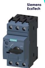
Special type Circuit breaker size S00 for motor protection, CLASS 10 A-release 10...16 A N-release 208 A screw terminal Standard switching capacity Ambient temperature -50  $^\circ$ C 500 switching cycles
