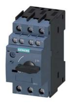
Circuit breaker size S00 for motor protection, Class 10 A-release 9...12 A N-release 163 A Screw terminal Standard switching capacity with transverse auxiliary switches 1 NO+1 NC Multi-unit packaging Pack = 12 units
