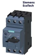
Circuit breaker size S00 for motor protection, CLASS 10 A-release 9...12 A N-release 163 A screw terminal Standard switching capacity
