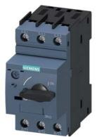
Circuit breaker size S00 for motor protection, CLASS 10 A-release 4.5...6.3 A N-release 82 A screw terminal Standard switching capacity Multi-unit packaging Pack = 24 units
