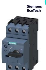
Special type Circuit breaker size S00 for motor protection, CLASS 10 A-release 4.5...6.3 A N-release 82 A screw terminal Standard switching capacity Ambient temperature -50  $^\circ$ C 500 switching cycles
