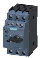
Circuit breaker size S00 for motor protection, CLASS 10 A-release 3.5...5 A N release 65 A screw terminal Standard switching capacity with transverse auxiliary switches 1 NO+1 NC Multi-unit packaging Pack = 12 units
