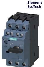
Special type Circuit breaker size S00 for motor protection, CLASS 10 A-release 3.5...5 A N release 65 A screw terminal Standard switching capacity with transverse auxiliary switches 1 NO+1 NC Ambient temperature -50  $^\circ$ C 500 switching cycles
