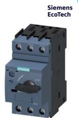
Special type Circuit breaker size S00 for motor protection, CLASS 10 A-release 3.5...5 A N release 65 A screw terminal Standard switching capacity Ambient temperature -50  $^\circ$ C 500 switching cycles
