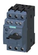
Special type Circuit breaker size S00 for motor protection, CLASS 10 A-release 2.8...4 A N release 52 A screw terminal Standard switching capacity with transverse auxiliary switches 1 NO+1 NC Ambient temperature -50  $^{\circ}\text{C}$  500 switching cycles
