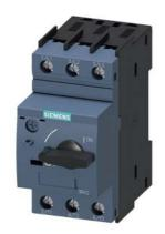
Circuit breaker size S00 for motor protection, CLASS 10 A-release 2.8...4 A N release 52 A screw terminal Standard switching capacity Multi-unit packaging Pack = 24 units
