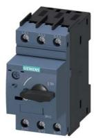
Special type Circuit breaker size S00 for motor protection, CLASS 10 A-release 2.2...3.2 A N release 42 A screw terminal Standard switching capacity Ambient temperature -50  $^\circ$ C 500 switching cycles
