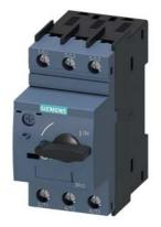
Circuit breaker size S00 for motor protection, CLASS 10 A-release 1.8...2.5 A N-release 33 A screw terminal Standard switching capacity Reusable packaging Pack = 43 units
