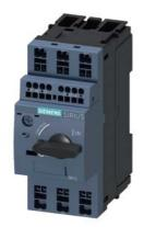
Circuit breaker size S00 for motor protection, CLASS 10 A-release 1.4...2 A N-release 26 A Spring-type terminal Standard switching capacity with transverse auxiliary switches 1 NO+1 NC
