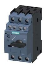
Circuit breaker size S00 for motor protection, Class 10 A-release 1.4...2 A N-release 26 A Screw terminal Standard switching capacity with transverse auxiliary switches 1 NO+1 NC Multi-unit packaging Pack = 12 units
