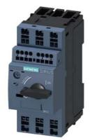
Circuit breaker size S00 for motor protection, CLASS 10 A-release 1.1...1.6 A N-release 21 A Spring-type terminal Standard switching capacity with transverse auxiliary switches 1 NO+1 NC  $\,$
