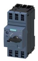
Circuit breaker size S00 for motor protection, CLASS 10 A-release 0.9...1.25 A N-release 16 A Spring-type terminal Standard switching capacity
