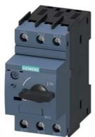
Circuit breaker size S00 for motor protection, CLASS 10 A-release 0.9...1.25 A N-release 16 A screw terminal Standard switching capacity Multi-unit packaging Pack = 24 units
