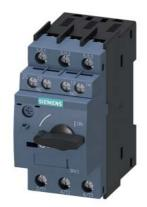
Circuit breaker size S00 for motor protection, CLASS 10 A-release 0.7...1 A N-release 13 A screw terminal Standard switching capacity with transverse auxiliary switches 1 NO+1 NC
