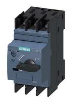
Circuit breaker size S00 for motor protection, CLASS 10 A-release 0.55...0.8 A N-release 10 A ring cable lug connection Standard switching capacity
