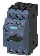
Circuit breaker size S00 for motor protection, CLASS 10 A-release 0.35...0.5 A N-release 6.5 A screw terminal Standard switching capacity with transverse auxiliary switches 1 NO+1 NC
