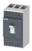
Molded case circuit breaker 3RV1 for starter combination Standard switching capacity Rated current In = 250 A electronic release Short-circuit protection adjustable 1-10 x In Icu = 120 kA at 400 V 3-pole, Screw terminal including phase barriers
