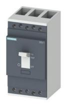
Molded case circuit breaker 3RV1 for motor protection Standard switching capacity Rated current In = 200 A electronic release Short-circuit protection adjustable 6-13 x In Overload protection adjustable 0.4-1 x In, Class 10A-32 Icu = 120 kA at 400 V 3-pole, Screw terminal including phase barriers
