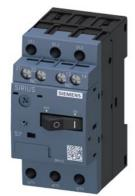
Circuit breaker size S00 for motor protection, CLASS 10 A-release 1.8...2.5 A N-release 33 A Screw terminal Standard switching capacity with transverse auxiliary switch 1 NO+1 NC
