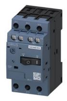
Circuit breaker size S00 for motor protection, CLASS 10 A-release 0.55...0.8 A N-release 10 A Screw terminal Standard switching capacity with transverse auxiliary switch 1 NO+1 NC
