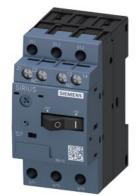
Circuit breaker size S00 for motor protection, CLASS 10 A-release 0.28...0.4 A N-release 5.2 A Screw terminal Standard switching capacity with transverse auxiliary switch 1 NO+1 NC
