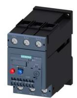
Overload relay 47...57 A Thermal For motor protection Size S2, Class 10 Standalone installation Main circuit: Screw Auxiliary circuit: spring-type terminal Manual-Automatic-Reset
