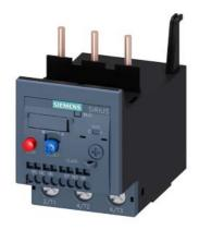
Overload relay 62...73 A Thermal For motor protection Size S2, Class 10A Contactor mounting Main circuit: Screw Auxiliary circuit: spring-type terminal Manual-Automatic-Reset
