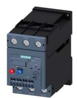
Overload relay 54...65 A Thermal For motor protection Size S2, Class 10 Standalone installation Main circuit: Screw Auxiliary circuit: spring-type terminal Manual-Automatic-Reset
