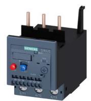
Overload relay 40... 50 A Thermal For motor protection Size S2, Class 10 Contactor mounting Main circuit: Screw Auxiliary circuit: spring-type terminal Manual-Automatic-Reset
