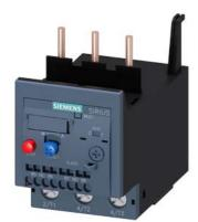
Overload relay 28...40 A Thermal For motor protection Size S2, Class 10 Contactor mounting Main circuit: Screw Auxiliary circuit: spring-type terminal Manual-Automatic-Reset
