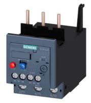
Overload relay 22...32 A Thermal For motor protection Size S2, Class 10 Contactor mounting Main circuit: Screw Auxiliary circuit: Screw Manual-Automatic-Reset
