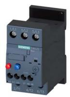
Overload relay 23...28 A Thermal For motor protection Size S0, Class 10 Standalone installation Main circuit: Screw Auxiliary circuit: Screw Manual-Automatic-Reset
