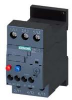
Overload relay 17...22 A Thermal For motor protection Size S0, Class 10 Standalone installation Main circuit: Screw Auxiliary circuit: Screw Manual-Automatic-Reset
