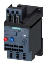
Overload relay 3.5...5.0 A Thermal For motor protection Size S00, Class 10 Standalone installation Main circuit: Spring-type terminal Auxiliary circuit: spring-type terminal Manual-Automatic-Reset
