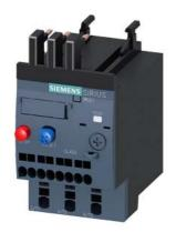
Overload relay 2.8...4.0 A Thermal For motor protection Size S00, Class 10 Contactor mounting Main circuit: Spring-type terminal Auxiliary circuit: spring-type terminal Manual-Automatic-Reset
